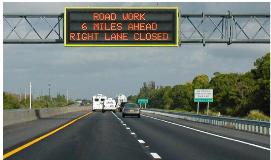
Example of a variable message sign
